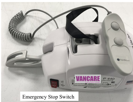
Figure 14C –RED Emergency stop switch located on the front left side of the lift.
