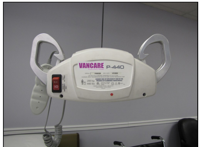
Figure 17B - P-440 (303073) with extended hooks (637045) turned upwards.
