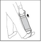
Test the FlexiMove regularly by stepping on one handle and pulling hard on one of the handles on the opposite side. Repeat the procedure until all of the handles have been tested.
