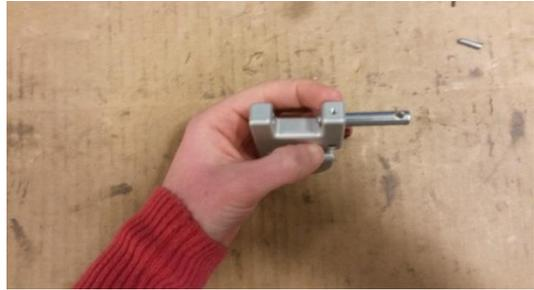
**Step 3)** Insert the pin back through the lift's strap. Tighten the set screw.
