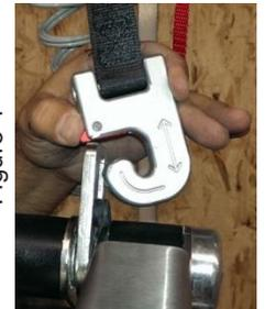
**Step 4)** Detach the QRS Hook from the attachment point on the **Independent Lifter** (see Figure 4).
