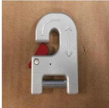
**Step 2)** Using a 2.5 mm Allen Key, loosen the set screw of the quick release hook and remove the pin.
