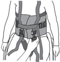
2. The leg cuffs are fastened at one of the three optional connections that is closest to being centered over the hip joint.
